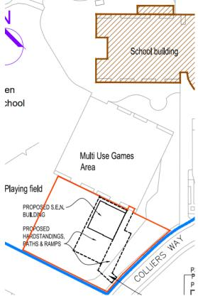
Extract from 'Proposed Site Plan Showing Development Area' (Dwg no 5924/A004 rev P3) showing location of proposed building and access onto Colliers Way.
